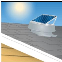
Roof ventilation is an important aspect of maintaining the structure of your home as well as saving energy. Improper roof venting can lead to moisture buildup that can cause mould growth and also cause wood rot. The key to proper roof ventilation is to create continuous air circulation throughout the roof space while preventing moisture from entering. In an ideal venting system, air should enter the roof from the eaves or soffits and escape outside at the roofs ridge.
